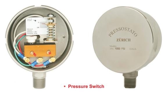
Using the technology "Bourdon," which consists in curved pipe in format "C" or helical, the model is characterized by high reliability, durability and high performance in processes - hydraulic, pneumatic, corrosive fluids, gases and liquids, constructed entirely in stainless steel, sensor, casing and parts in contact with fluid, the model ZPU ensures exceptional performance in environments chemically aggressive and hostile environments.
